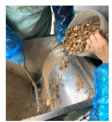
Figure 6. Shelling method: a blower separates the kernels from the shells
